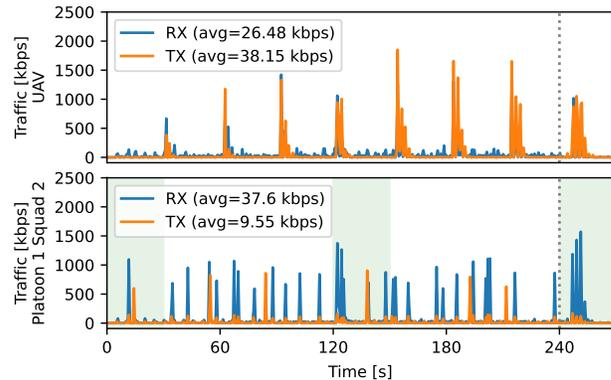
Fig. 6: Bandwidth utilization of the UAV and one representative squad, as observed during the evaluation.
