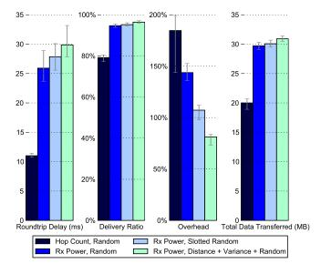
Fig. 4. A comparison of different distance and delay metrics.
