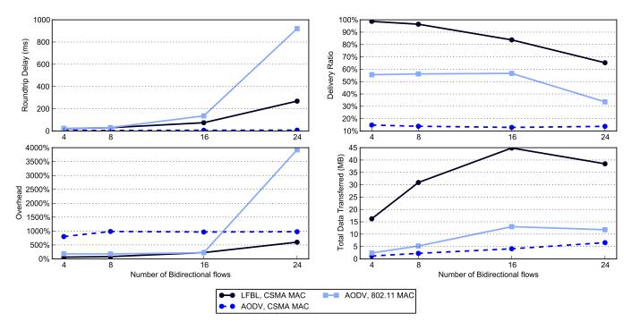
Fig. 2. Effect of the number of simultaneous data flows in the network.
